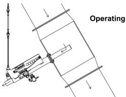
Once the unit is activated, the sample tube is inserted into the product flow by the use of an air cylinder. Product enters the sampler through a slotted opening in the sample tube and flows via gravity out of the sample discharge point. This process can be repeated as often as desired either automatically or manually.
