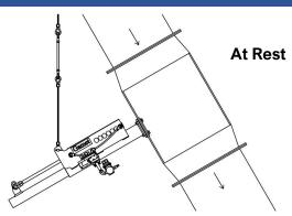
Between sampling cycles the B-310 stainless steel sampling tube is withdrawn from the product flow. This reduces sample tube wear and significantly increases the useful life of the sampler.
